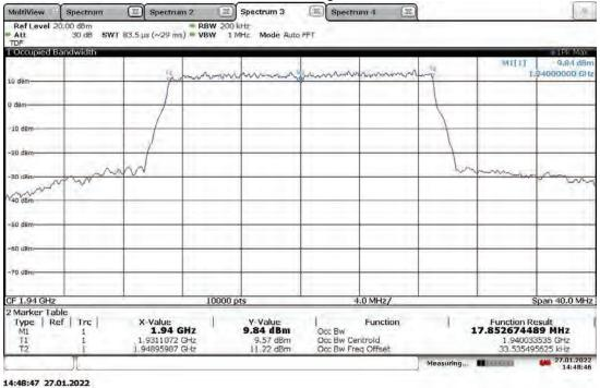
Slot 0 (Band 2), ANT1, Modulation: QPSK, Bandwidth: 20 MHz, High Channel 1980 MHz (5G nR) Lower Extreme Voltage: 41.1VDC
