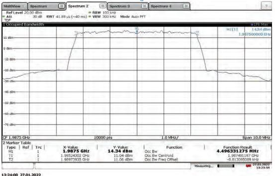
Slot 0 (Band 2), ANT1, Modulation: QPSK, Bandwidth: 5 MHz, Low Channel 1932.5 MHz (5G nR) Upper Extreme Voltage: 57.0VDC
