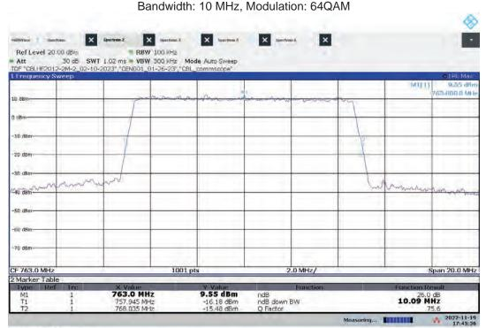
Lo-PIM – ANTO High Channel Emission/Band Edge (Mask e (1)) Bandwidth: 10 MHz, Modulation: 64QAM
