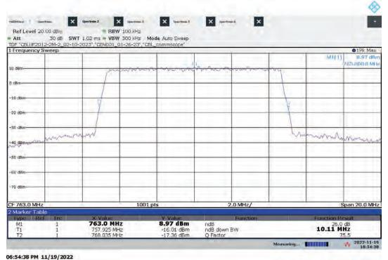
Hi-PIM – ANT1 High Channel 26 dB Bandwidth Bandwidth: 10 MHz, Modulation: 256QAM
