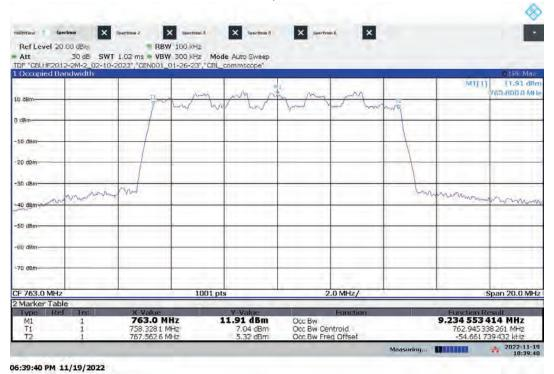
Hi-PIM – ANT1 High Channel Occupied Bandwidth Bandwidth: 10 MHz, Modulation: 16QAM
