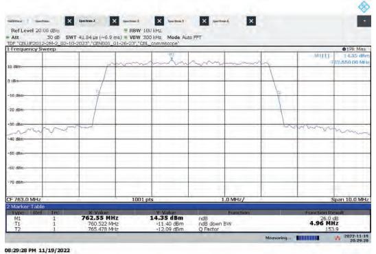
Hi-PIM – ANT1 Mid Channel 26 dB Bandwidth Bandwidth: 5 MHz, Modulation: 256QAM
