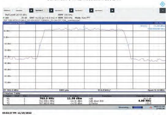
Lo-PIM – ANTO High Channel 26 dB Bandwidth Bandwidth: 10 MHz, Modulation: QPSK
