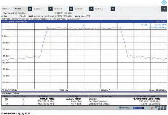
Hi-PIM – ANTO Mid Channel Occupied Bandwidth Bandwidth: 5 MHz, Modulation: QPSK
