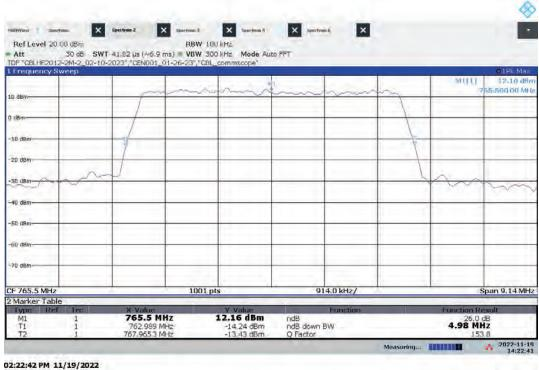
Lo-PIM – ANTO Low Channel 26 dB Bandwidth Bandwidth: 5 MHz, Modulation: 16QAM
