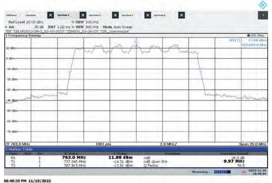
Hi-PIM – ANT1 High Channel 26 dB Bandwidth Bandwidth: 10 MHz, Modulation: 16QAM
