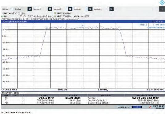
Hi-PIM – ANT0 Low Channel Occupied Bandwidth Bandwidth: 5 MHz, Modulation: 256QAM
