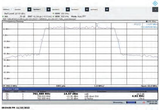
Hi-PIM – ANTO Mid Channel 26 dB Bandwidth Bandwidth: 5 MHz, Modulation: 64QAM
