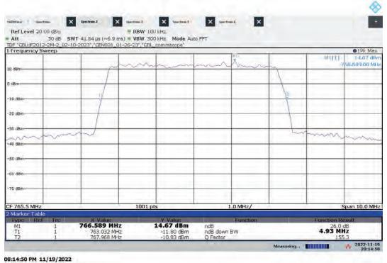
Hi-PIM – ANT1 High Channel 26 dB Bandwidth Bandwidth: 5 MHz, Modulation: 64QAM
