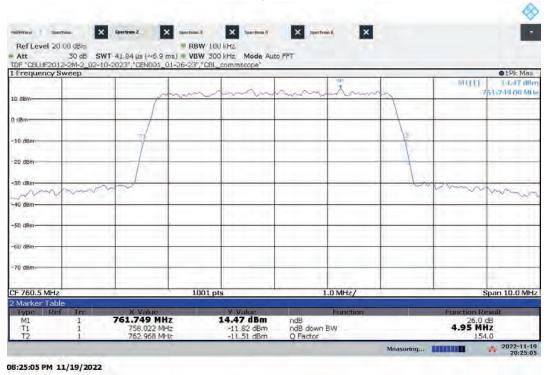
Hi-PIM – ANTO Mid Channel 26 dB Bandwidth Bandwidth: 5 MHz, Modulation: 256QAM
