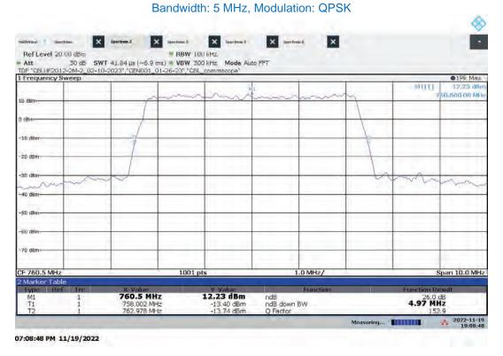
Hi-PIM – ANTO Mid Channel 26 dB Bandwidth Bandwidth: 5 MHz, Modulation: QPSK
