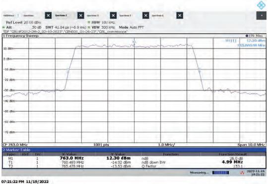
Hi-PIM - ANTO High Channel 26 dB Bandwidth Bandwidth: 5 MHz, Modulation: QPSK
