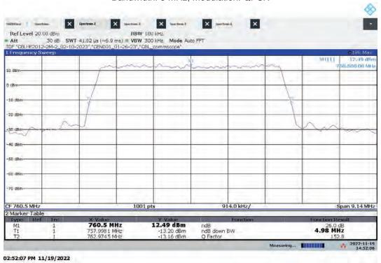
Lo-PIM – ANT0 Mid Channel 26 dB Bandwidth Bandwidth: 5 MHz, Modulation: QPSK
