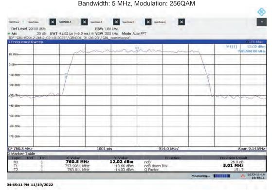
Lo-PIM - ANTO Mid Channel 26 dB Bandwidth Bandwidth: 5 MHz, Modulation: 256QAM
