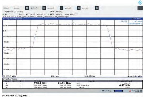
Lo-PIM – ANT1 High Channel 26 dB Bandwidth Bandwidth: 5 MHz, Modulation: 64QAM
