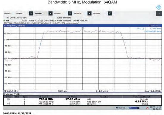
Lo-PIM – ANTO High Channel 26 dB Bandwidth Bandwidth: 5 MHz, Modulation: 64QAM
