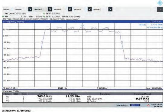
Lo-PIM – ANT1 High Channel 26 dB Bandwidth Bandwidth: 10 MHz, Modulation: 16QAM
