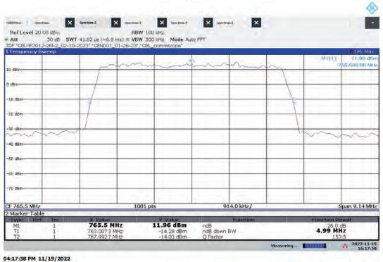
Lo-PIM – ANTO Low Channel 26 dB Bandwidth Bandwidth: 5 MHz, Modulation: 256QAM
