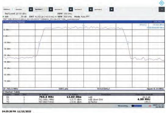
Lo-PIM – ANT1 High Channel 26 dB Bandwidth Bandwidth: 5 MHz, Modulation: 256QAM
