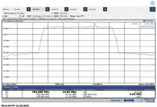
Hi-PIM – ANTO High Channel 26 dB Bandwidth Bandwidth: 5 MHz, Modulation: 64QAM
