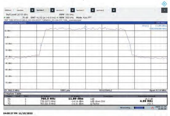
Lo-PIM – ANT0 Mid Channel 26 dB Bandwidth Bandwidth: 5 MHz, Modulation: 64QAM
