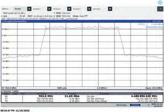
Hi-PIM - ANTO High Channel Occupied Bandwidth Bandwidth: 5 MHz, Modulation: 64QAM
