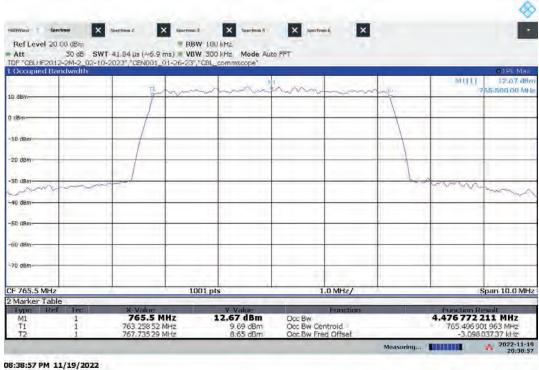
Hi-PIM – ANTO High Channel Occupied Bandwidth Bandwidth: 10 MHz, Modulation: QPSK
