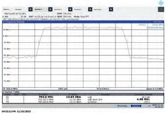
Lo-PIM - ANT1 Mid Channel 26 dB Bandwidth Bandwidth: 5 MHz, Modulation: 256QAM
