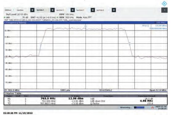
Lo-PIM - ANT1 High Channel 26 dB Bandwidth Bandwidth: 5 MHz, Modulation: QPSK
