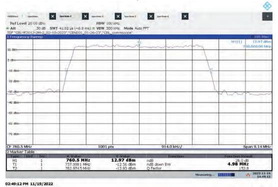
Lo-PIM – ANT1 Low Channel 26 dB Bandwidth Bandwidth: 5 MHz, Modulation: QPSK
