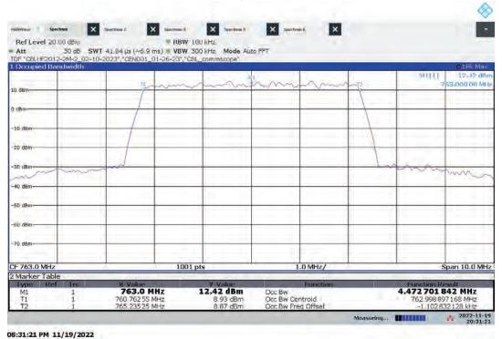
Hi-PIM - ANTO High Channel Occupied Bandwidth Bandwidth: 5 MHz, Modulation: 256QAM
