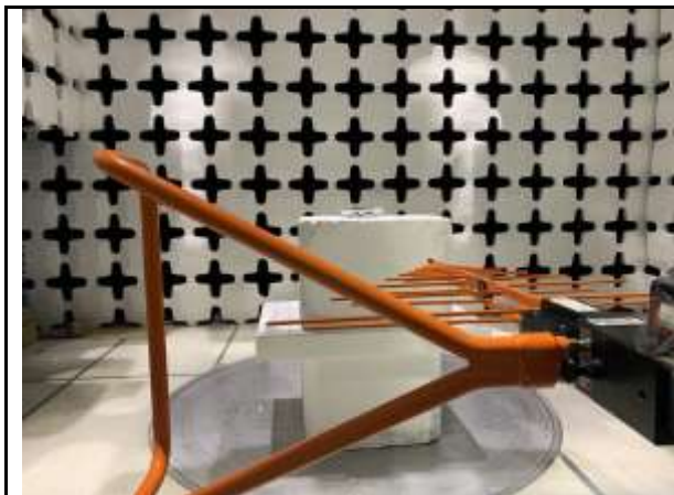
Radiated Emission Test below 1GHz Front View
