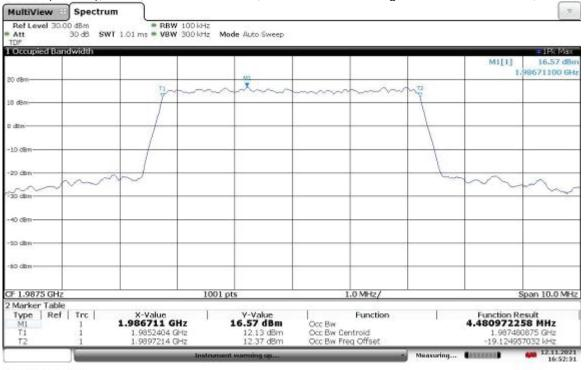
Slot 0 (Band 2), ANT1, Modulation: QPSK, Bandwidth: 5 MHz High Channel 1987.5 MHz, 10 °C
