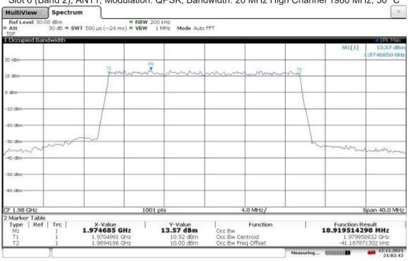
Slot 0 (Band 2), ANT1, Modulation: QPSK, Bandwidth: 20 MHz High Channel 1980 MHz, 30 °C
