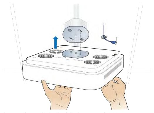
6 Secure the RP to the plate by twisting the RP counterclockwise.
