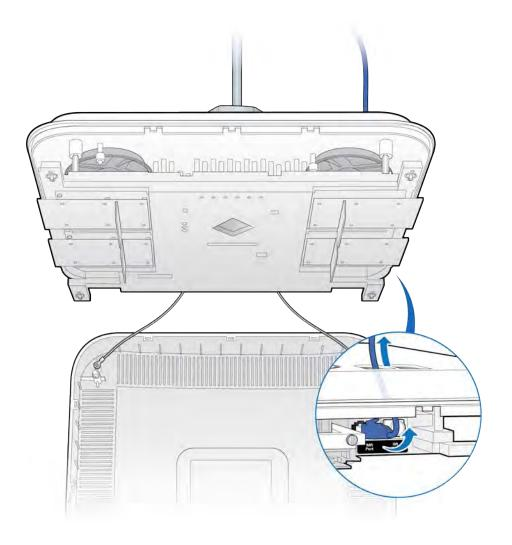
**3** Replace the cover and twist the RP clockwise.
