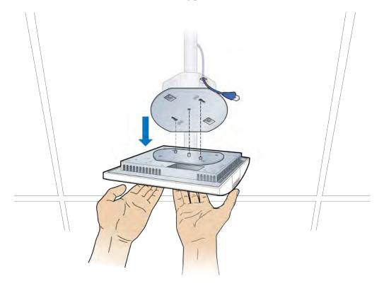
**5** Attach the plate to the replacement RP.
