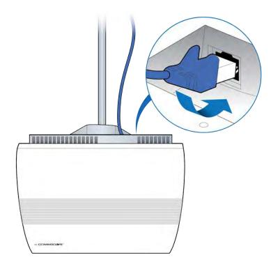
**8** Verify the RP installation. See The operational state of the RP can be determined by the LED status on the RP. Additional information can be attained from the WebGUI status screens.
