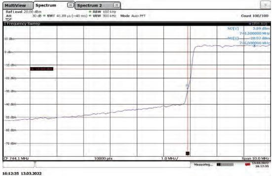
Band Edge Compliant, Lower Band Edge, 748.5 MHz (4G LTE) With RP5200 Host Slot 0 (Band 13), Antenna Port: ANT1, Bandwidth: 5 MHz, Modulation: TM3.1a-256QAM
