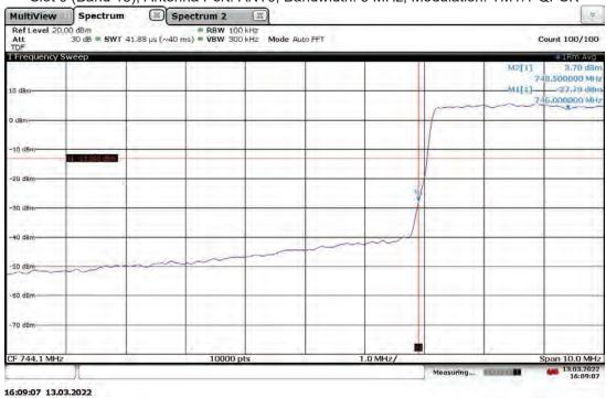
Band Edge Compliant, Lower Band Edge, 748.5 MHz (4G LTE) With RP5200 Host Slot 0 (Band 13), Antenna Port: ANT1, Bandwidth: 5 MHz, Modulation: TM1.1-QPSK
