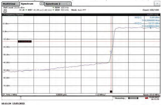
Band Edge Compliant, Lower Band Edge, 748.5 MHz (4G LTE) With RP5200 Host Slot 0 (Band 13), Antenna Port: ANT1, Bandwidth: 5 MHz, Modulation: TM3.1-64QAM
