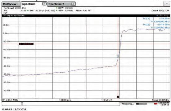
Band Edge Compliant, Lower Band Edge, 748.5 MHz (4G LTE) With RP5200 Host Slot 0 (Band 13), Antenna Port: ANT1, Bandwidth: 5 MHz, Modulation: TM3.2-16QAM
