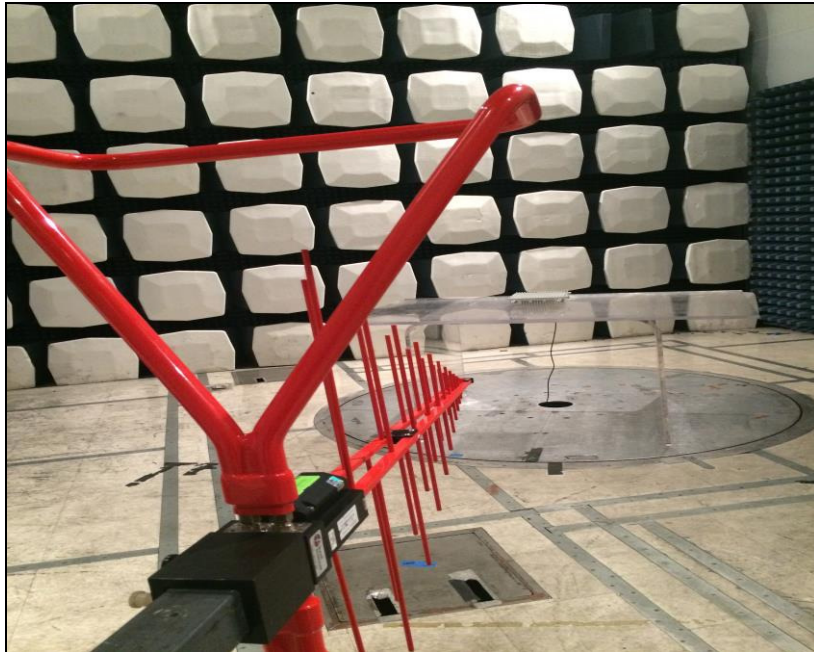
Photograph 1. Radiated Spurious Emissions 30 MHz – 1 GHz, Test Setup
