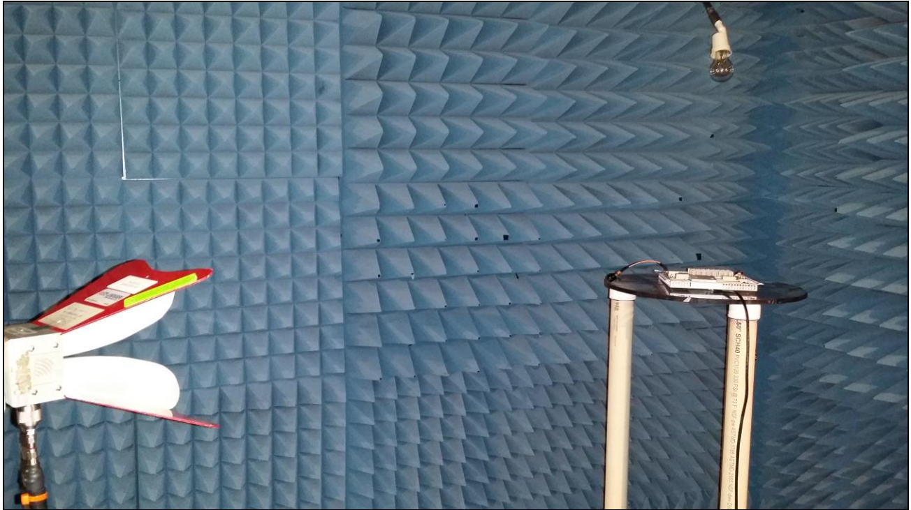
Photograph 1. Radiated Spurious Emissions, Above 1 GHz, Test Setup
