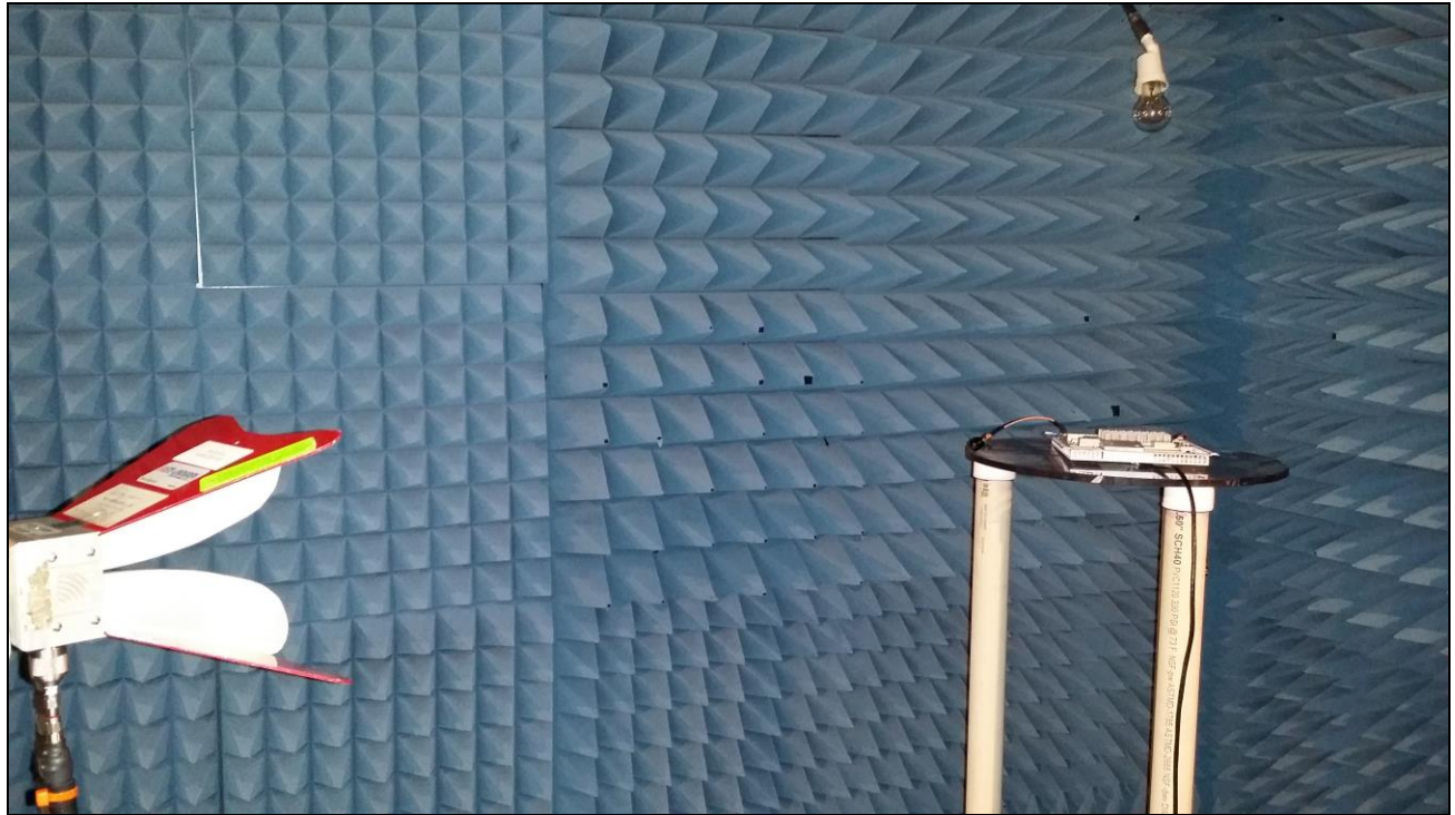
Photograph 1. Radiated Spurious Emissions above 1 GHz, Test Setup
