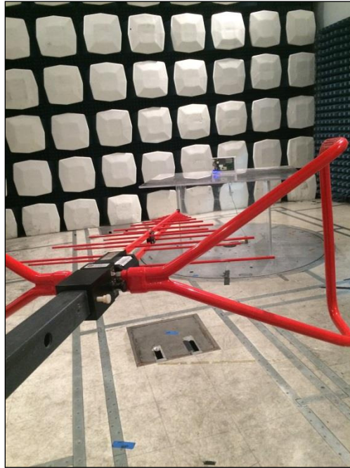
Photograph 1. Radiated Spurious Emissions, Test Setup, 30 MHz – 1 GHz
