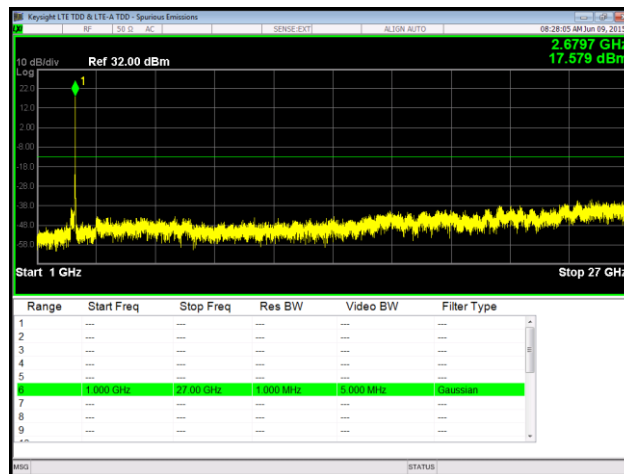
Plot 114. Spurious Emissions at Antenna Terminal, 64QAM, High Channel, Port 2, 1 GHz – 27 GHz
