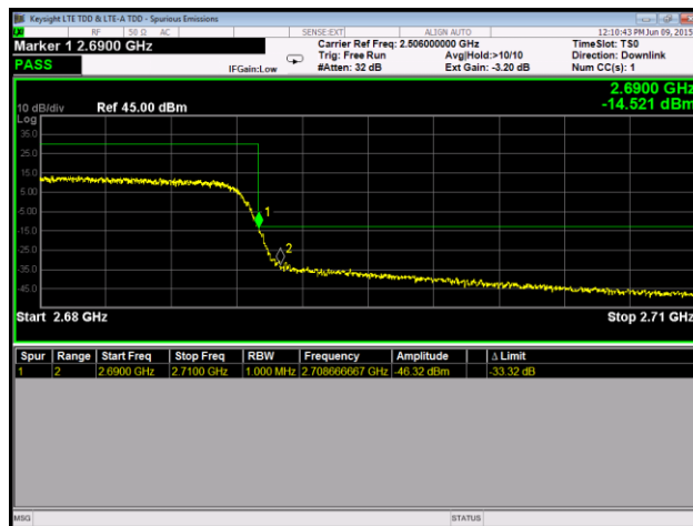
Plot 134. Conducted Band Edge, 64QAM, High Channel, Port 2
