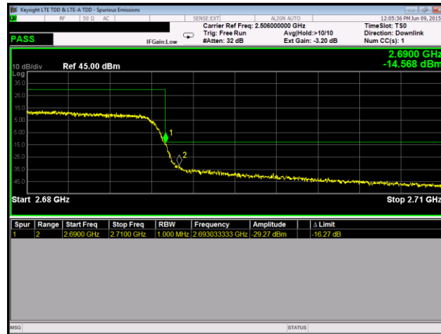
Plot 138. Conducted Band Edge, QPSK, High Channel, Port 2
