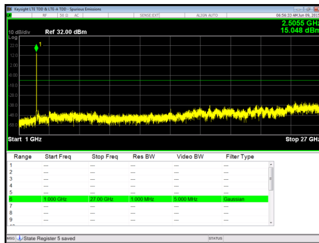
Plot 116. Spurious Emissions at Antenna Terminal, QPSK, Low Channel, Port 1, 1 GHz – 27 GHz
