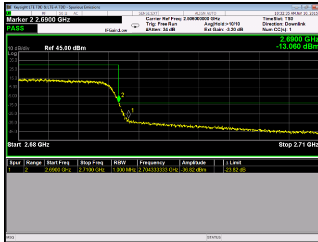
Plot 146. Frequency Stability, QPSK, High Channel, Port 1, 10°C
