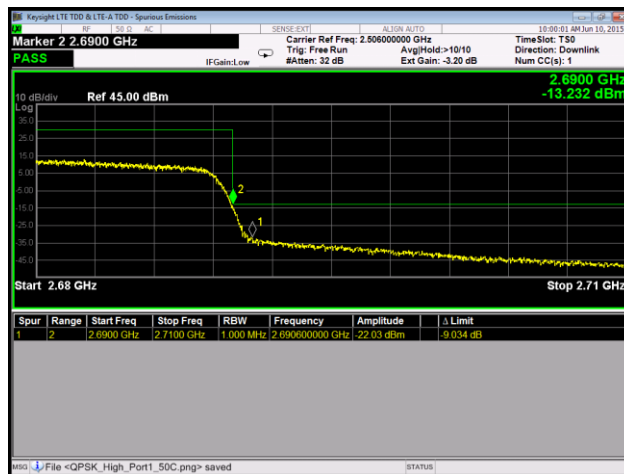
Plot 148. Frequency Stability, QPSK, High Channel, Port 1, 40°C
