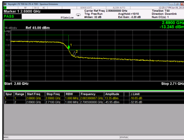
Plot 132. Conducted Band Edge, 64QAM, High Channel, Port 1
