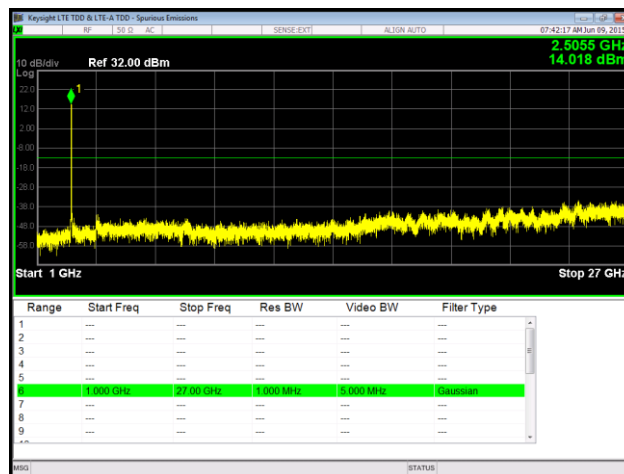
Plot 92. Spurious Emissions at Antenna Terminal, 16QAM, Low Channel, Port 1, 1 GHz – 27 GHz
