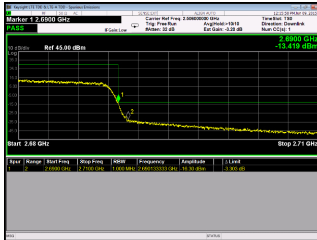
Plot 130. Conducted Band Edge, 16QAM, High Channel, Port 2
