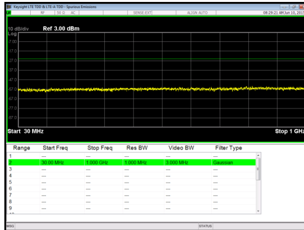
Plot 89. Spurious Emissions at Antenna Terminal, QPSK, Mid Channel, Port 2, 30 MHz – 1 GHz, RBW
