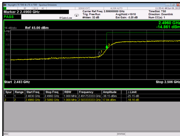
Plot 131. Conducted Band Edge, 64QAM, Low Channel, Port 1
