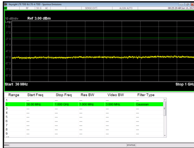
Plot 76. Spurious Emissions at Antenna Terminal, 16QAM, Low Channel, Port 2, 30 MHz – 1 GHz, RBW
