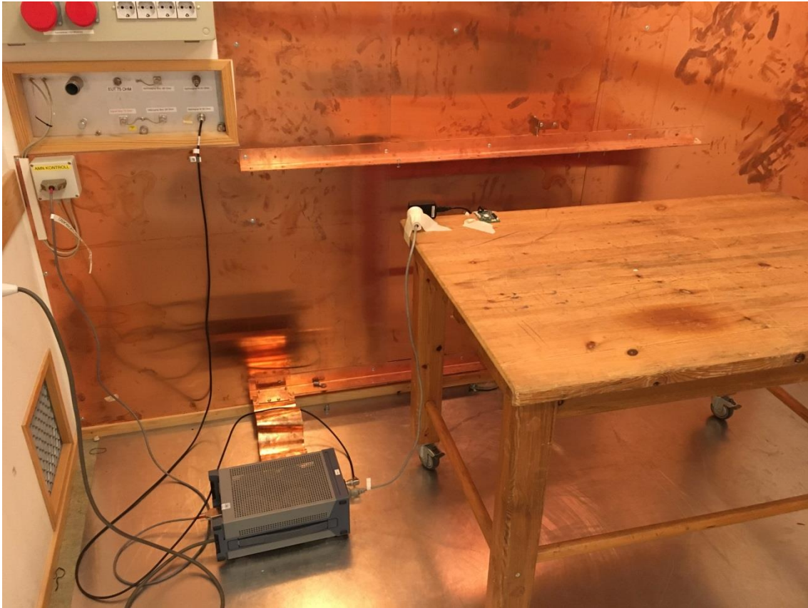
Test setup conducted continuous disturbances 9 kHz to 30 MHz
