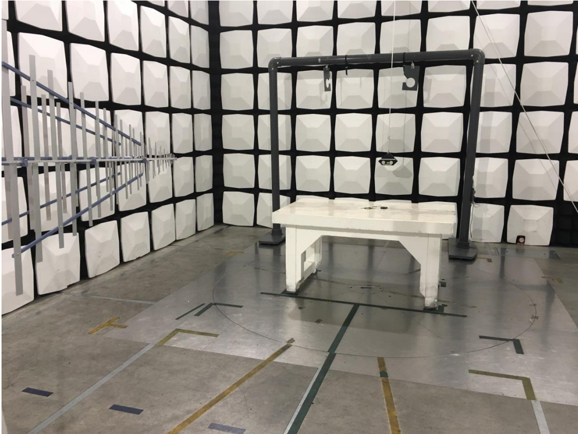
Test set up radiated emission 30 MHz – 1GHz
