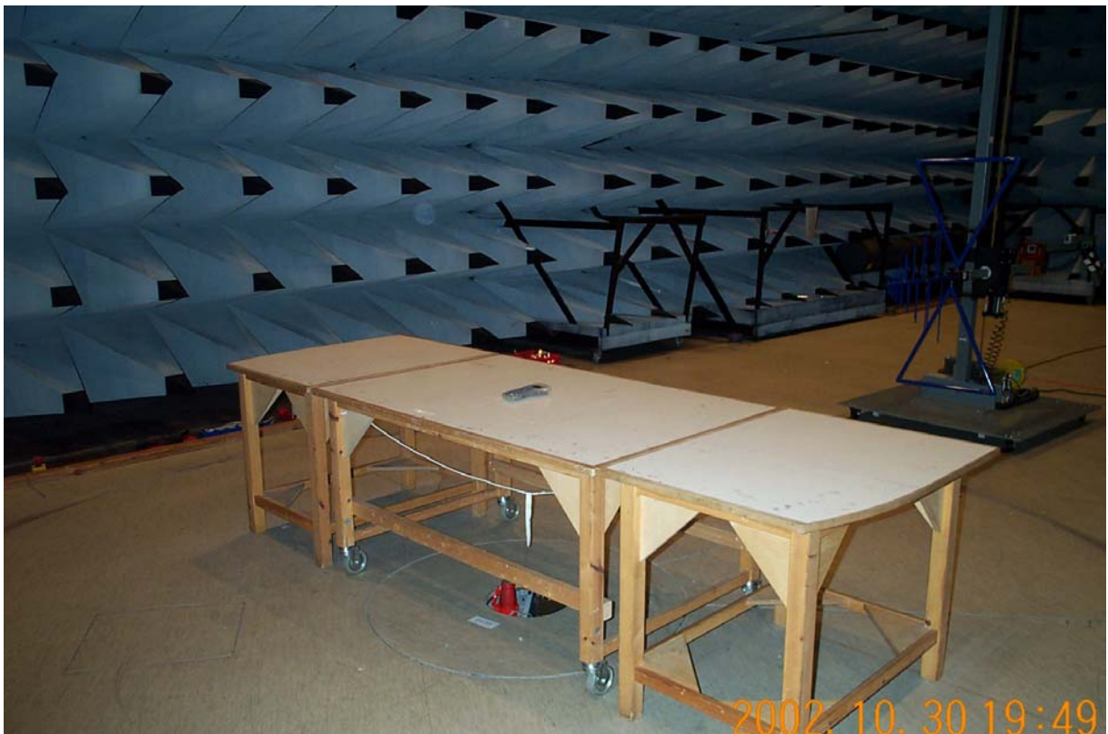
Photo 2 Set-up for measurements 30 - 1000 MHz.
