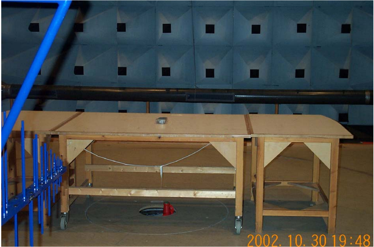
Photo 1 Set-up for measurements 30 - 1000 MHz
