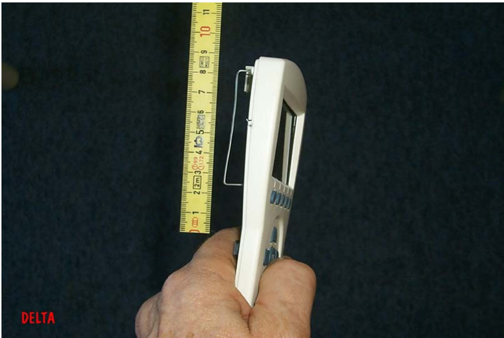
Distance between antenna and hand during normal operation is larger than 2,5 cm.
