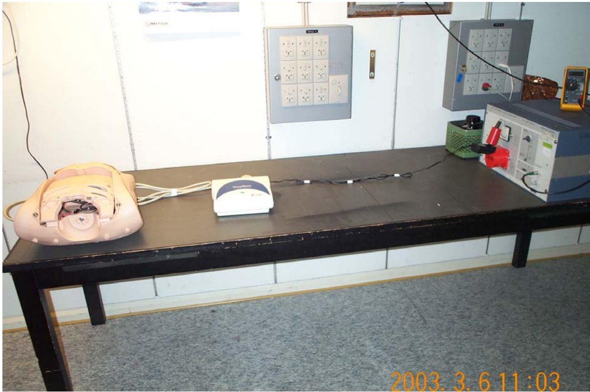
Test set-up Conducted emission, 0.15-30 MHz
