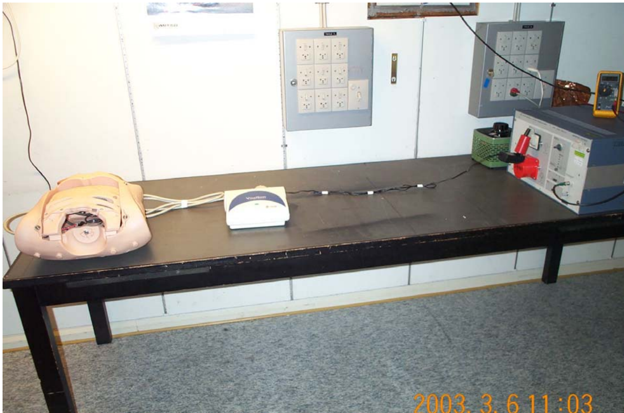
Test set-up. Conducted emission, 0.15-30 MHz
