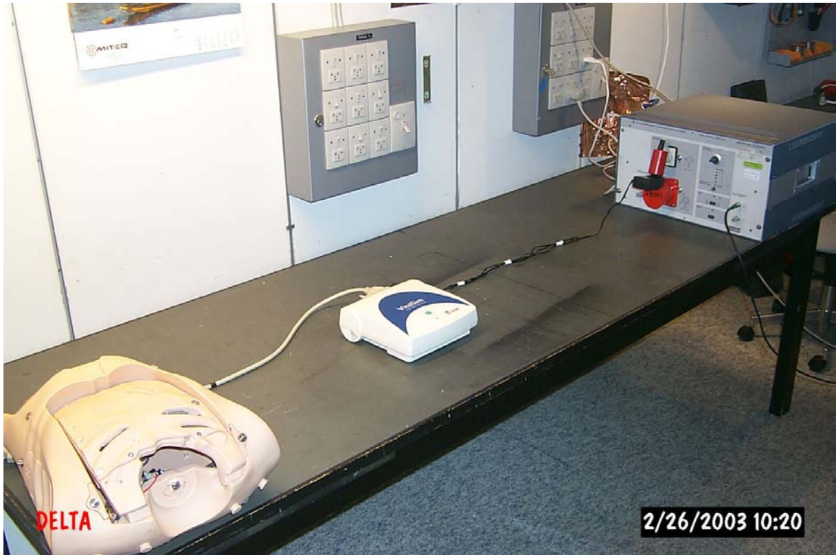
Photo 1 Set-up for measurements of conducted emission.
