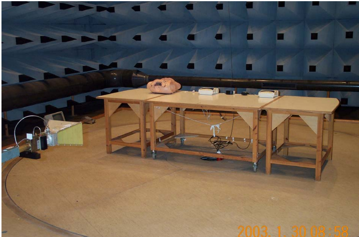
Photo 3 Set-up for measurements 1 - 10 GHz. One unit in Tx-mode and one in Rx-mode.
