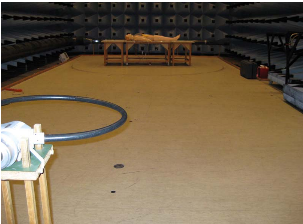
Photo 4.3.2 Test setup regarding measurement of radio frequency electromagnetic field.
