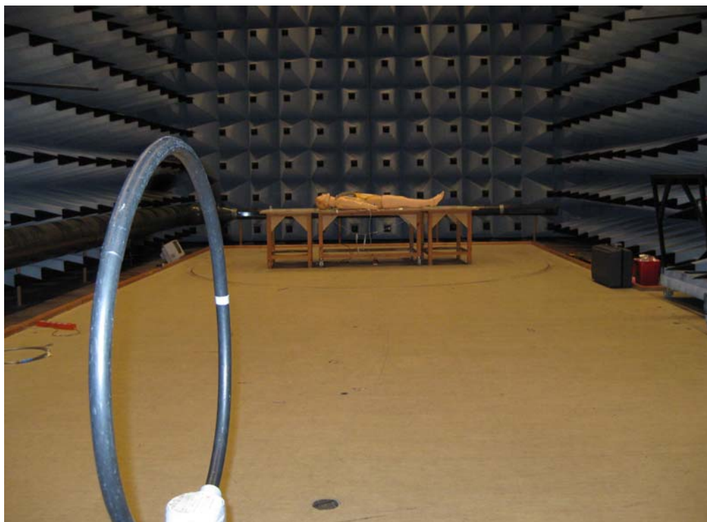
Photo 4.10.1 Test setup regarding measurement of radio frequency electromagnetic field.
