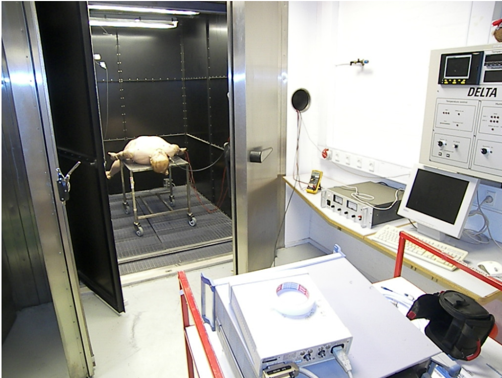
Photo 4.11.1 Test setup regarding measurement of frequency tolerance.
