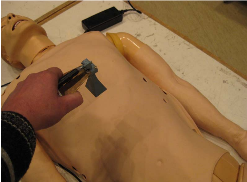
Photo 4.8.1 Test setup regarding measurement of radio frequency electromagnetic field.
