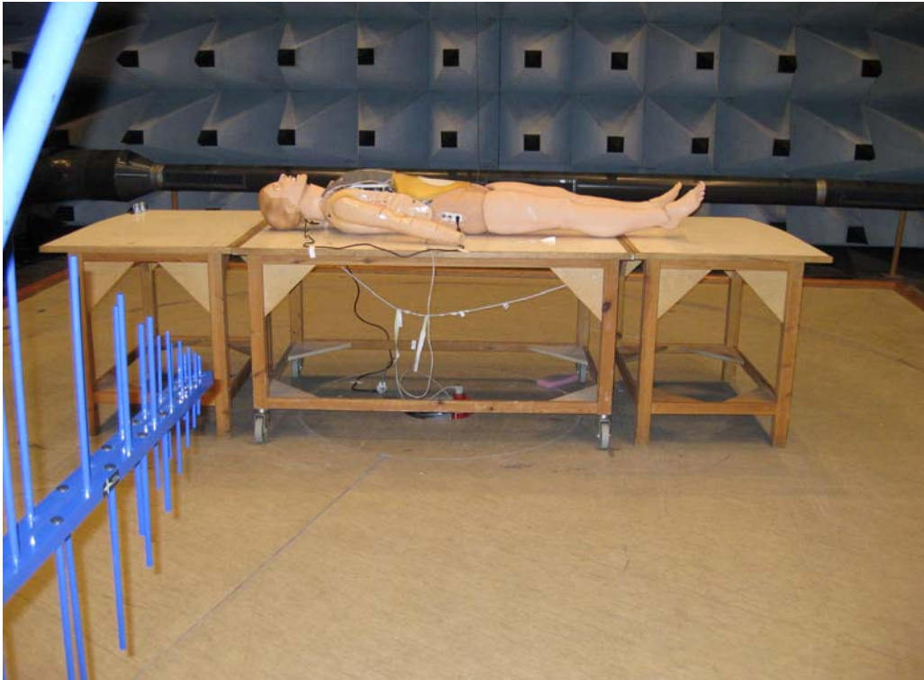
Photo 4.4.1 Test setup regarding measurement of radio frequency electromagnetic field.
