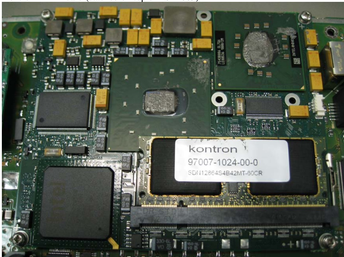
SAPS Base Board Kontron ETX Board (stacked on top of FST1009)
