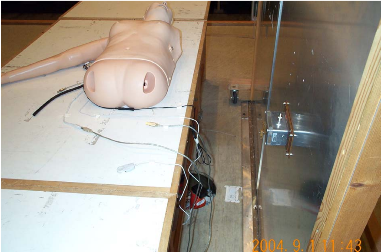
Photo A2.1 Test setup for conducted emission measurements.
