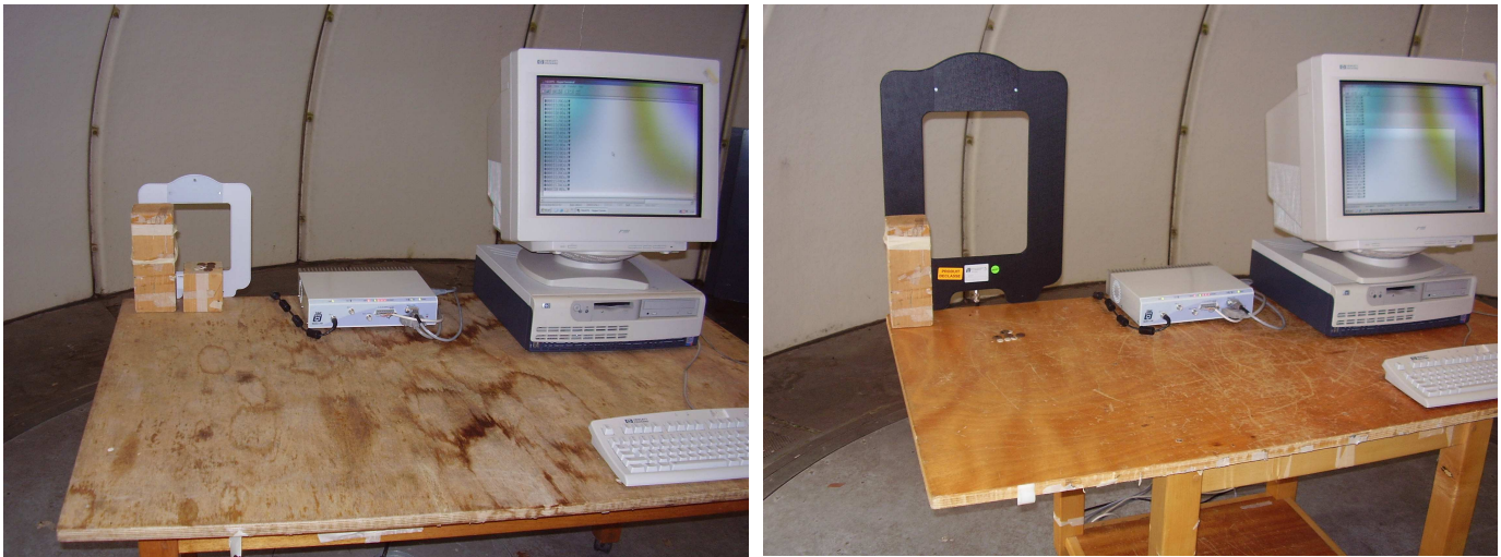
Radiated emission test setup (AERO-LB and AERO-LC antennas, in vertical position)
