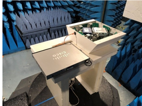
Test setup in anechoic chamber <1GHz
