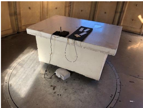
Test setup in anechoic chamber >1GHz (pre-characterization and characterization)
