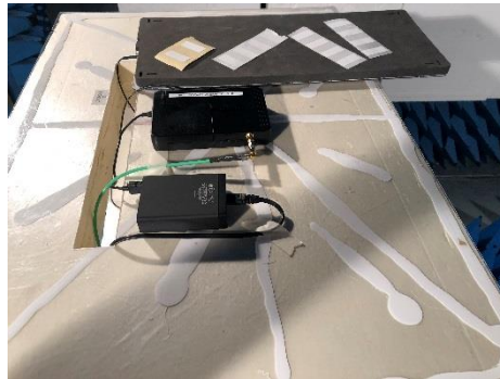
Test setup in anechoic chamber >1GHz (pre-characterization and characterization)
