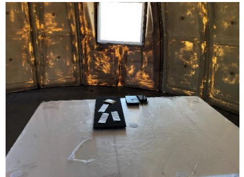
Test setup in anechoic chamber >1GHz (pre-characterization and characterization)
