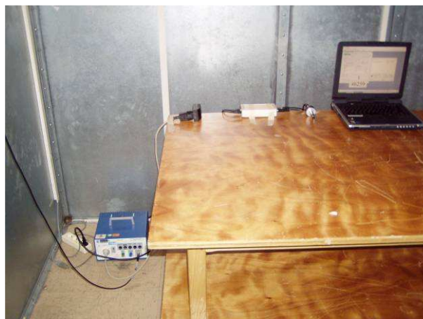
Dummy load (50Ω) replacing the antenna at the end of the cable
