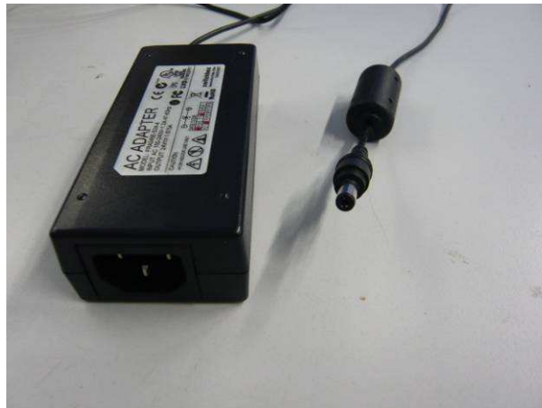
Detail views of SwitchBox power supply
