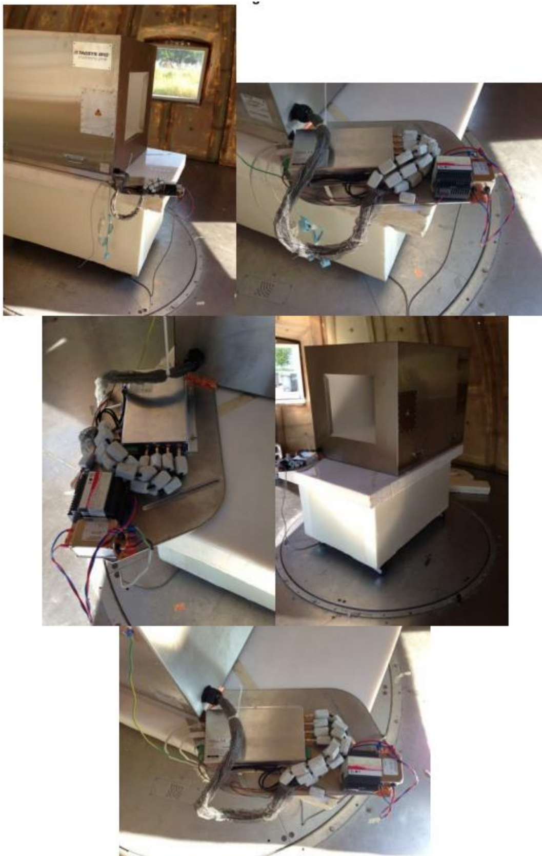
TUNNEL Antenna – Configuration n°2
