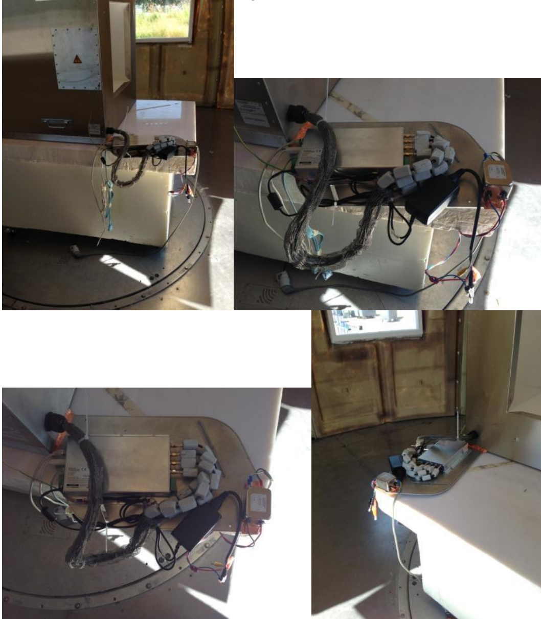
Radiated emission test setup
