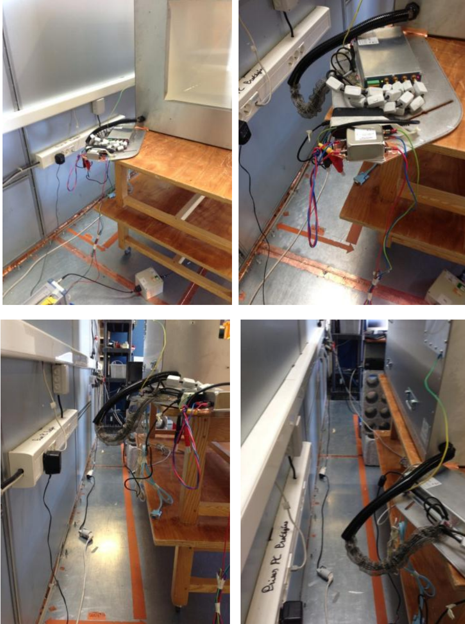
Conducted emission test setup
