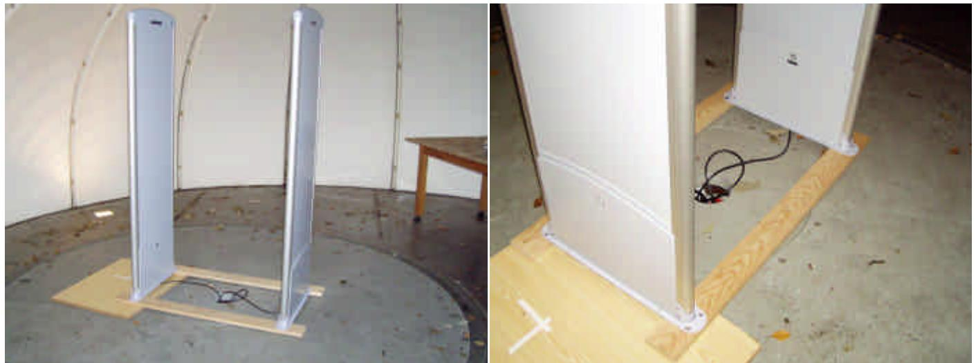
The installation of EUT is identical for pre-characterization measurement in a 3 meters full anechoic chamber and for measures on a 3 meters Open site.
