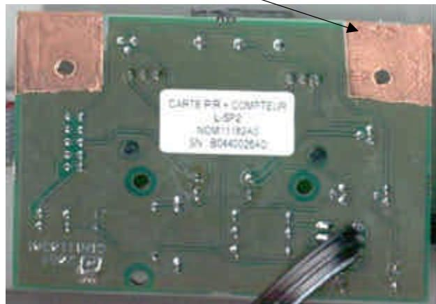
For production unit the sticky tape will be replaced by a copper plan on the PWB.
