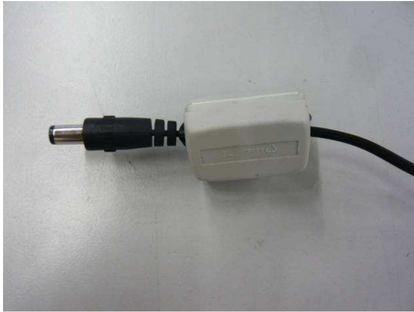
Detail views of connector with or without ferrite (WE 742 711 1, 2ways)
