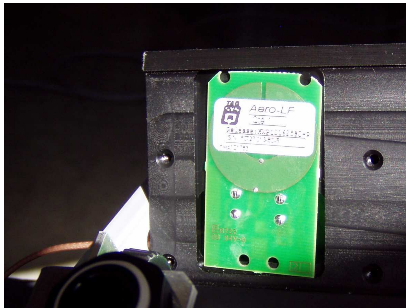
RF antenna placement (cover removed)
