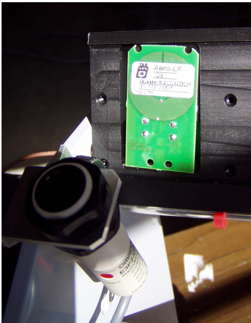
RF antenna placement
