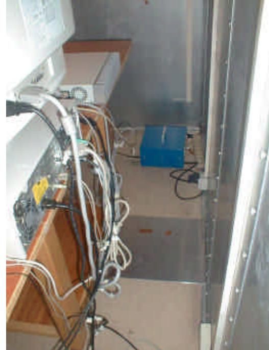
The MEDIO-L100 and PC are placed on a non-conducting table of 80cm height. The antenna support is set on the floor (isolated). The cable of the power supply (MEDIO-L100) has been shorted to 1 meter length. The MEDIO-L100 is powered through the LISN.
