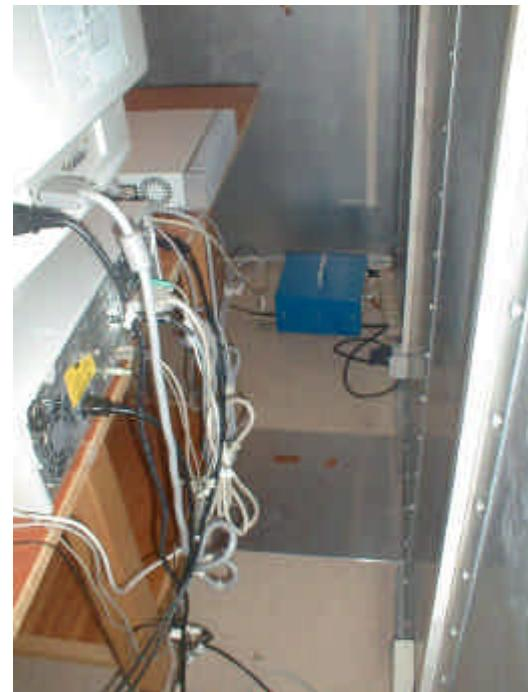
The MEDIO-L100 and PC are placed on a non-conducting table of 80cm height. The cable of the power supply (MEDIO-L100) has been shorted to 1 meter length. The MEDIO-L100 is powered through the LISN.
