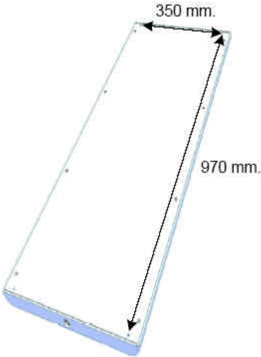
Figure 8: Conveyor Antenna Mechanical Diagram (Mounting Hole Dimensions)
