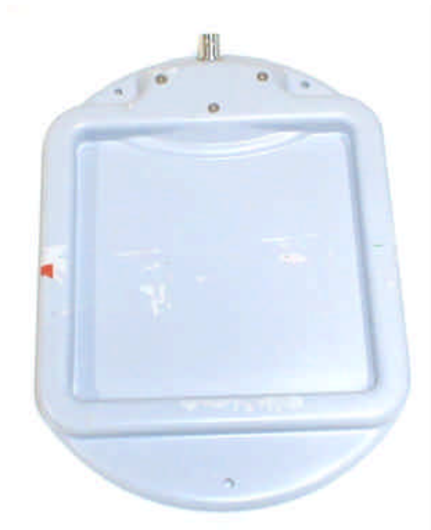
View of 140x140 antenna (font & rear face)
