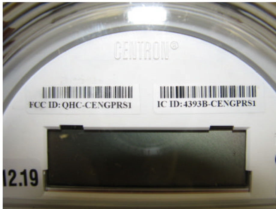
Figure 2: FCC and IC Label Examples – Located Above LCD Display
