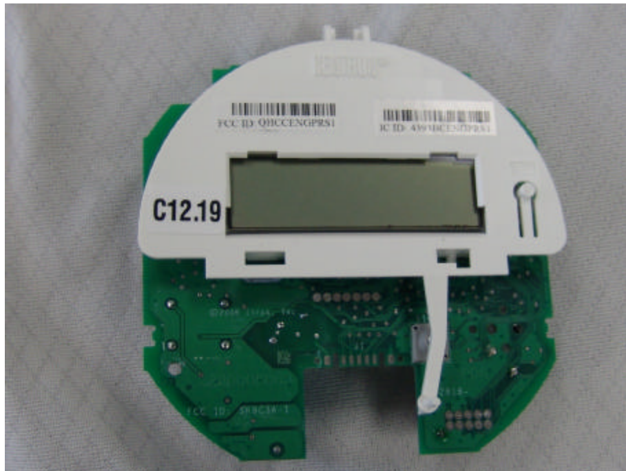
Figure 7: Itron Register and Display Board – Front View
