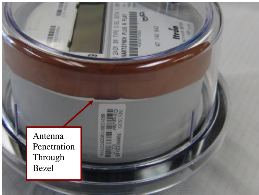
Figure 3: Flexible Dipole Antenna Location
