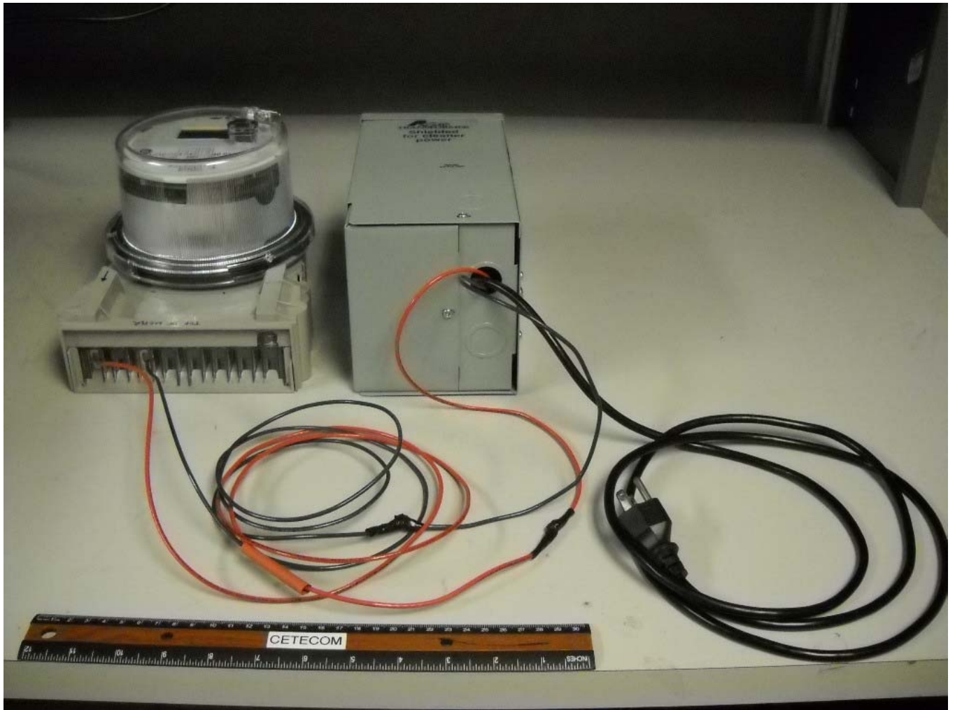
EUT and Power Transformer
