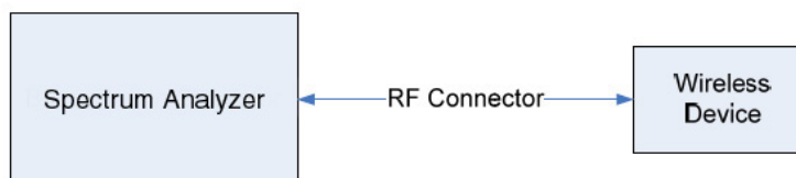
Figure 6-2. Test Instrument & Measurement Setup
