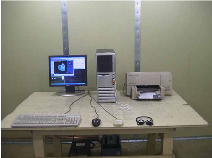
Photograph 2 : Setup for Conducted Emissions
