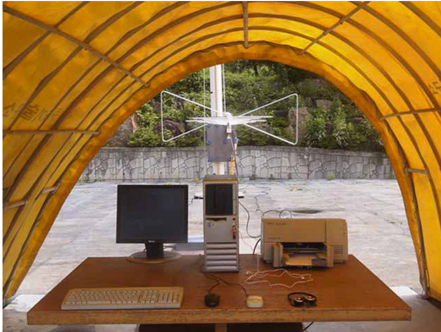
Photograph 1 : Setup for radiated Emissions
