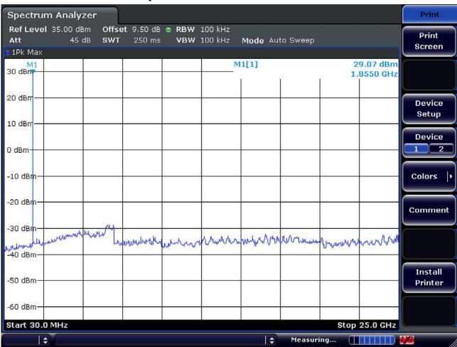
PCS1900 Spurious Emissions at Antenna Terminal / Ch.512
