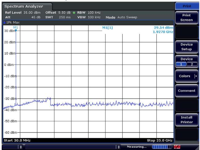
PCS1900 Spurious Emissions at Antenna Terminal / Ch.810
