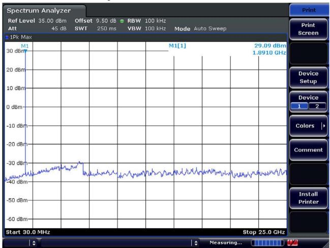
PCS1900 Spurious Emissions at Antenna Terminal / Ch.661
