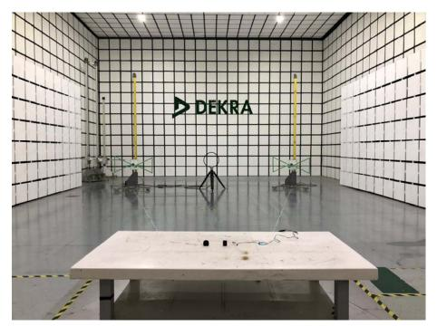
Description: Radiated Emission Test Setup for 30MHz~1000MHz
