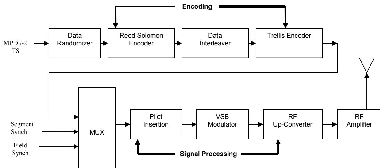
The first byte (sync byte) of the MPEG-2 data packet is stripped and the remaining 187 bytes are randomized using a polynomial generator to prevent long strings of fixed states (1 or 0) that may occur and could increase chances of error.
