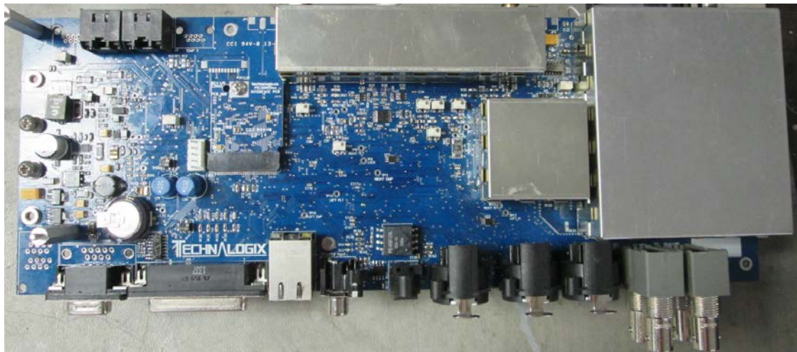
FM Exciter Construction (top):
