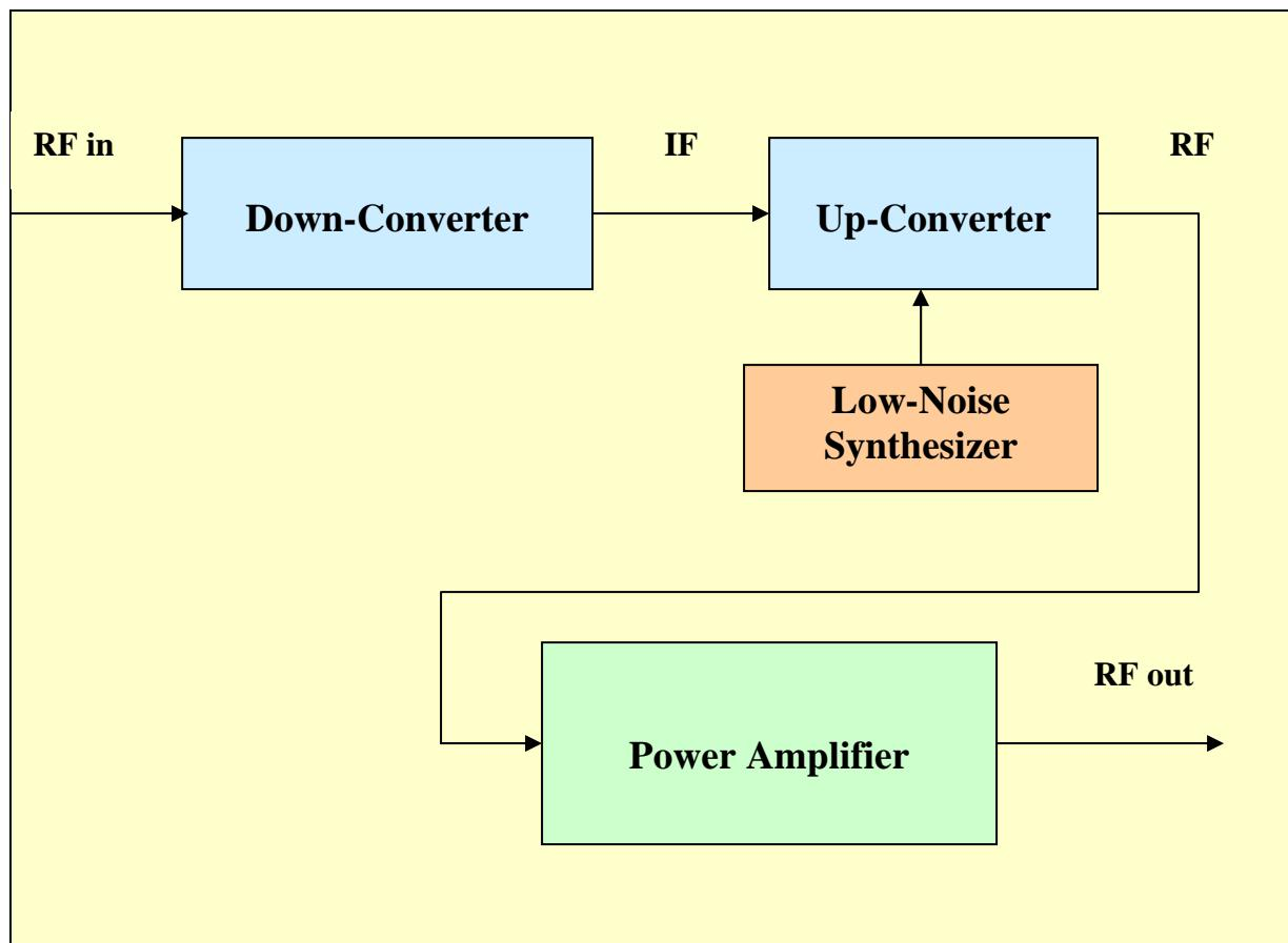
The first stage is the Down-Converter and it brings the frequency down to an IF signal. Then the 44MHz IF enters the UP-Converter which has an internal Low-Noise Synthesizer and it up-converts the IF to desired RF channel.
