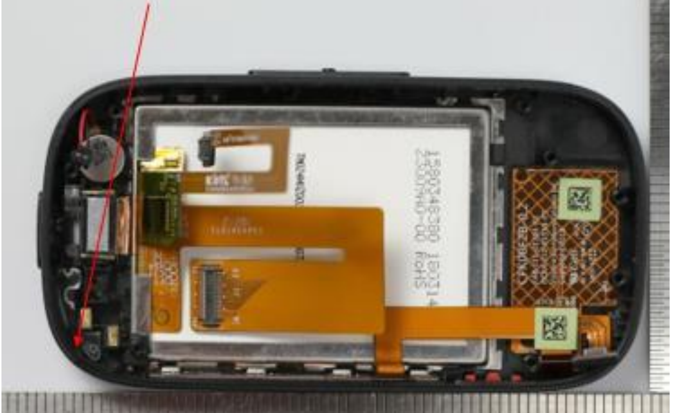
Pic. 2 Front cover with LCD display
