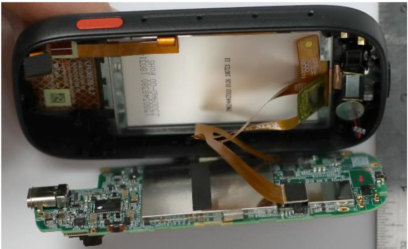
connection between LCD display and main board
