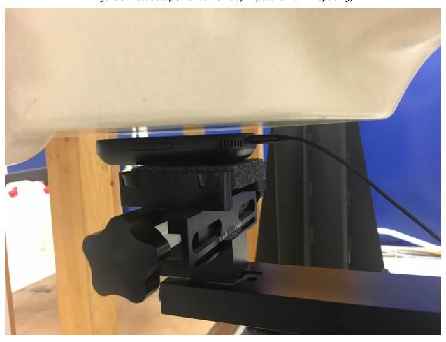
Figure 6: Test Setup (Back Side Body Exposure-5mm Spacing)
