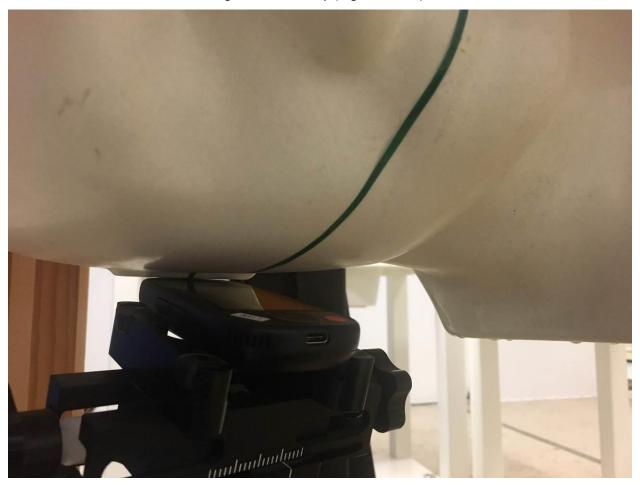
Figure 5: Test Setup (Front Side Body Exposure – 5mm Spacing)
