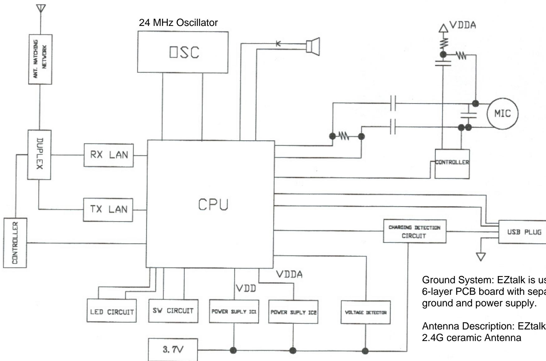
Ground System: EZtalk is using 6-layer PCB board with separate ground and power supply.
